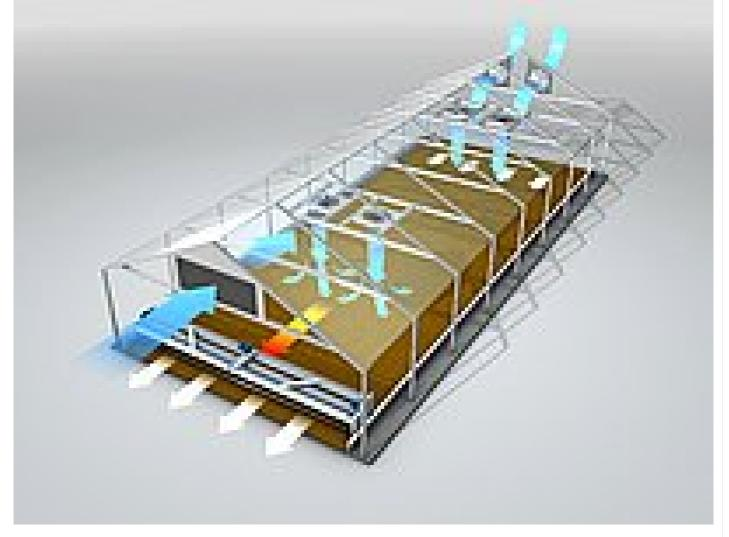
Water evaporation requires 800 - 900 kWh/t heat. Little heat is recovered. Sludge dryers also consume power.
