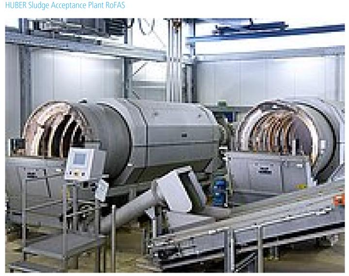
Wash drum for efficient and reliable coarse material separation for septic sludge
