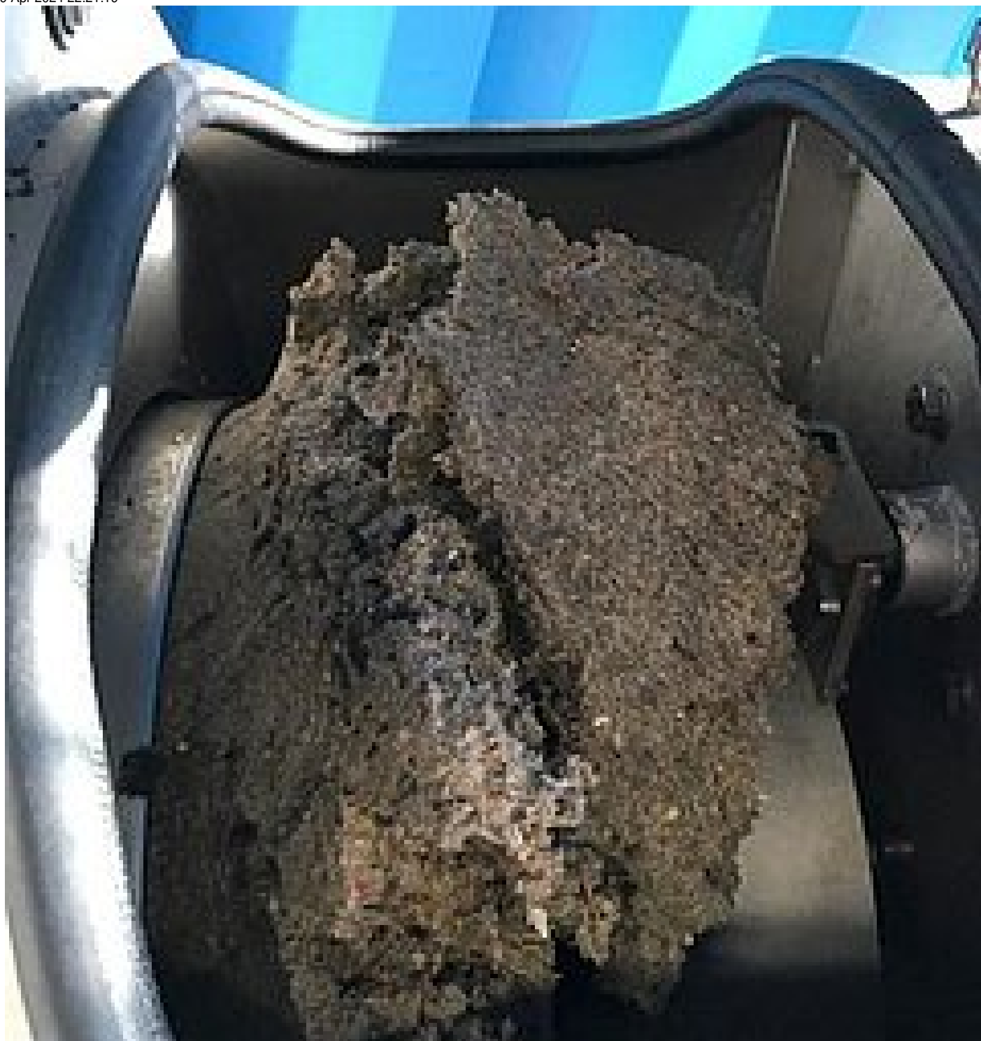
Fig. 5: Mechanically dewatered thin sludge from the HUBER Drum Screen LIQUID demo unit in a HUBER Screw Press Q-PRESS®
