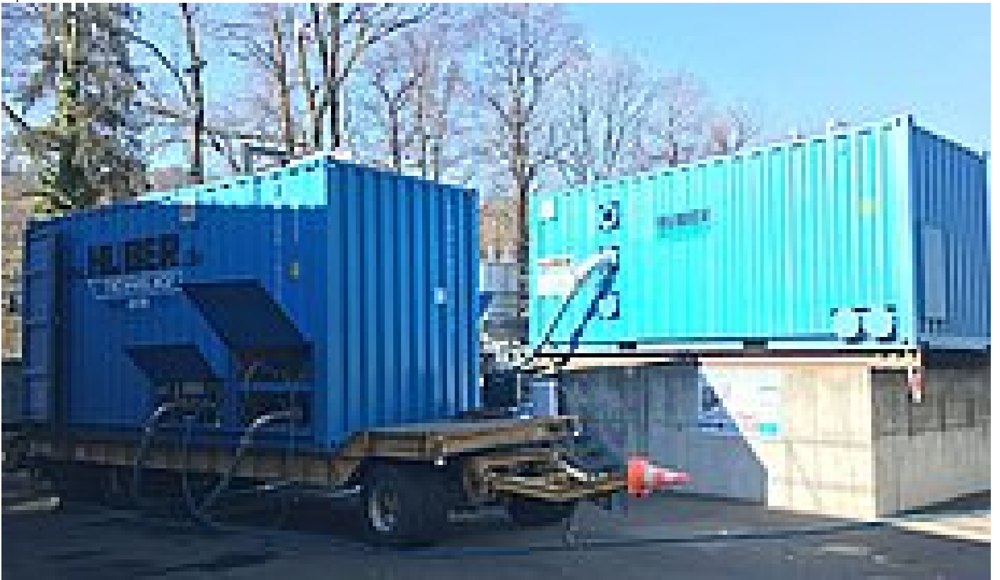
Fig. 4 Validation operation - HUBER Drum Screen LIQUID demo unit (right container) combined with the HUBER Screw Press Q-PRESS® demo unit (left container)
