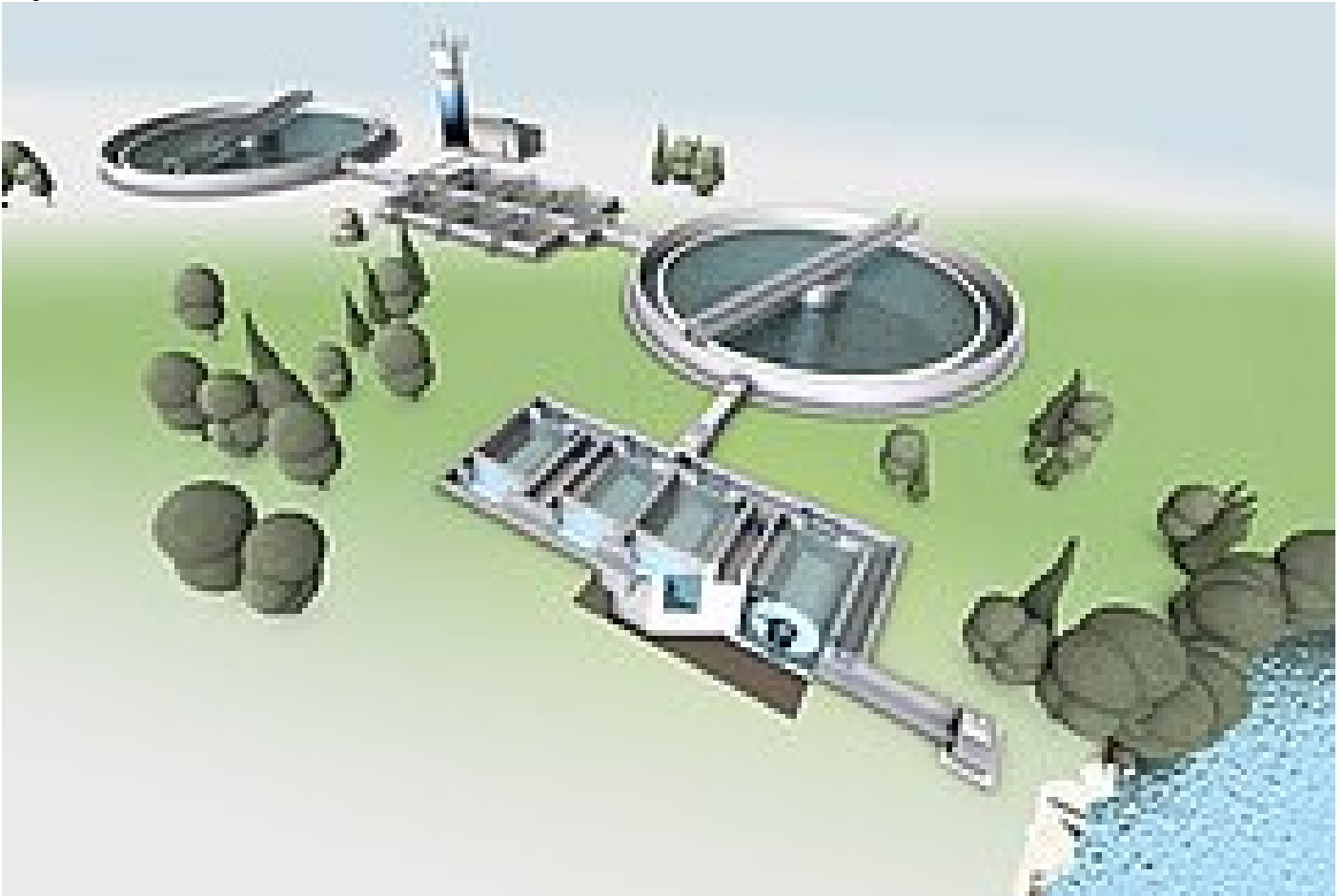
PAC process ("Ulm process") with downstream HUBER Disc Filter RotaFilt® as polishing filter
