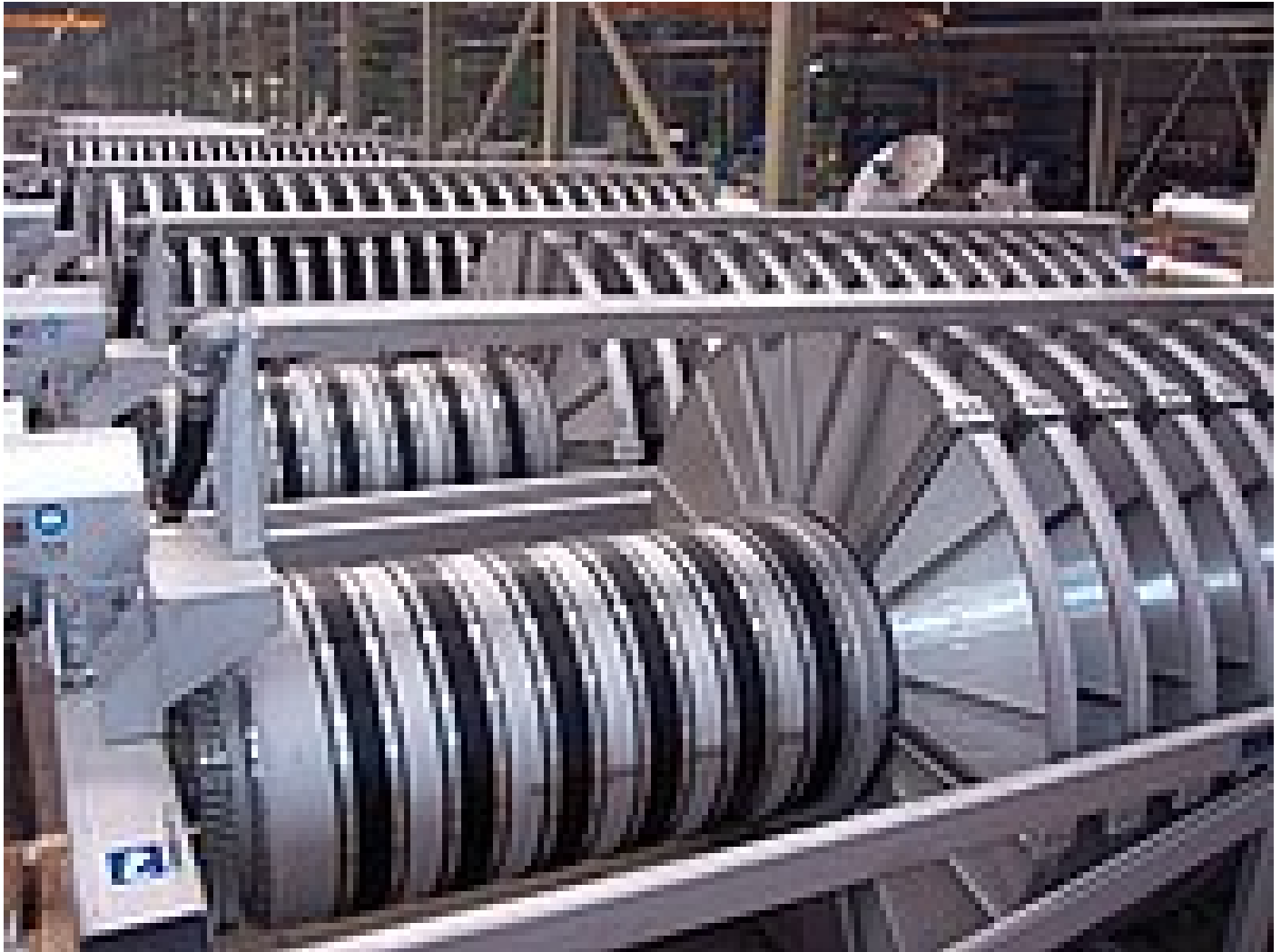
RoDisc® Micro-Strainers in the HUBER factory shortly before they were shipped to China
