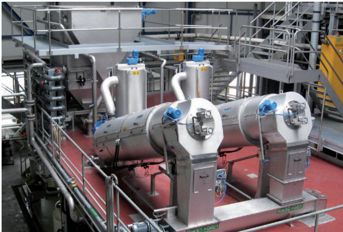
ROTAMAT® Screw Press RoS 3 units and HUBER Dissolved Air Flotation Plant HDF 5 with chemical treatment stage
