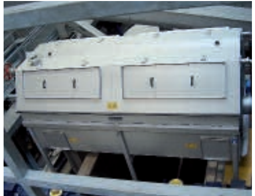
ROTAMAT® Rotary Drum Screen RoMesh® with 0.2 to 1.0 mm mesh
