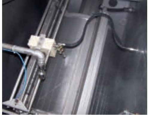
HUBER ROTAMAT® Rotary Drum Fine Screen Ro 2 with 1 mm bar spacing and moveable high pressure cleaning system
