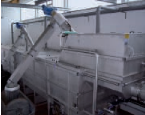
Complete mechanical wastewater treatment in a single and compact unit
