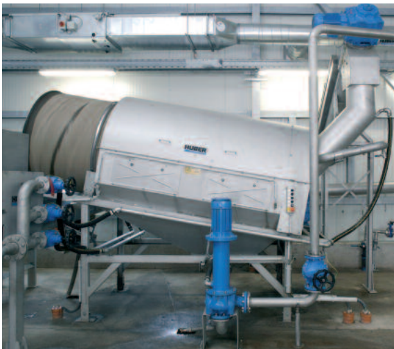
ROTAMAT® Wash Drum for washout and separation of all coarse material > 3/8" (10 mm)
