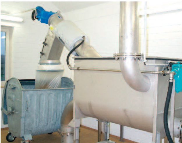
Tank-mounted ROTAMAT® Rotary Drum Fine Screen Ro 2 ...
